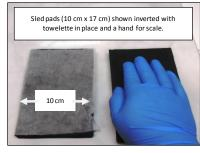
Sled construction: each towelette contacts the tile with identical surface area with matching force from the weights transmitted through a metal platen and a flexible elastomer pad which presses it onto the tile surface. Sleds are not attached to each other or the pusher arm.
